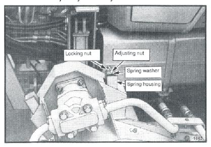
For standard cut on the mechanically driven rear flail mower, adjust so that the spring washer is flush with the spring guide as shown below.
